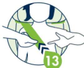
13 Grab the diagonal belt and pull towards the retractor to remove slack from the lap belt.
