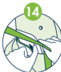
**14** Push the locking mechanism of the shoulder belt guide inwards and slide the three-point belt out of the belt guide.
