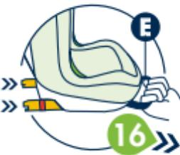
**16** Push the ISOFIX connectors back into the seat while pulling on the strap on the front (**E**) and then remove the seat from the vehicle.
