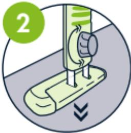
**2** Rotate the beautiful gray knob in a counter-clockwise direction. Pull out the leg's foot until it reaches the vehicle's floor. Once the height is defined, secure the position by tightening the knob in a clockwise direction. Talking about clocks... what time is it? Yes, it's happy o'clock!
