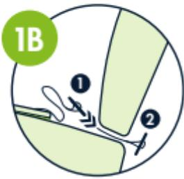
**1B** If the seat is not equipped with ISOFIX connectors: Please open the webbings, remove the hooks, and replace them with the anchor plates found in the included envelope. Slide them all the way through in between the backrest and the sitting cushion of the seat. Smooth!
