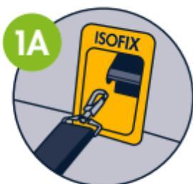
**1A** If the seat where you are installing the footrest is equipped with ISOFIX connections: Please hook the hooks on the ISOFIX anchorage points. Now dance the dance!
